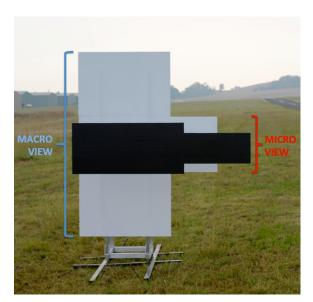
Macro vs. Micro View: This picture helps illustrate the more sensitive 'Micro View' in which, in this example, the approach would be slightly HIGHER than the glideslope at which the device has been set
